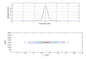
The upper panel is the cross-section and bottom is the couture plot of the corresponding ambiguity function
