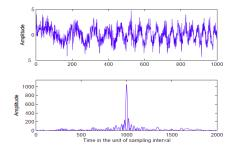
(The signal with white noise and its corresponding matched filter)
